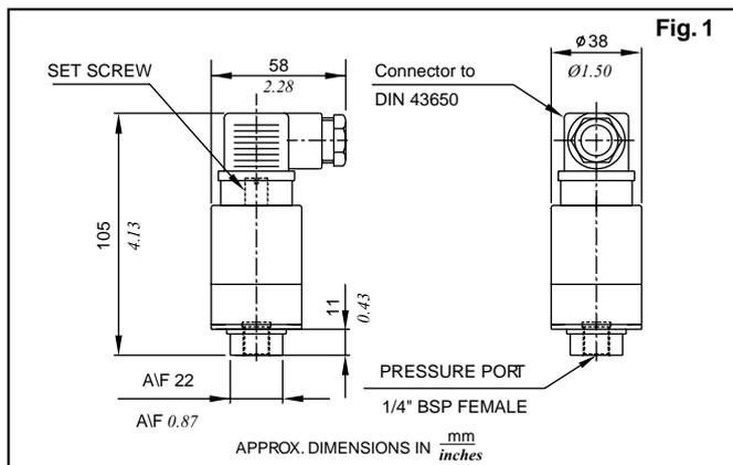
The SA model pressure switches can be mounted in any direction.
